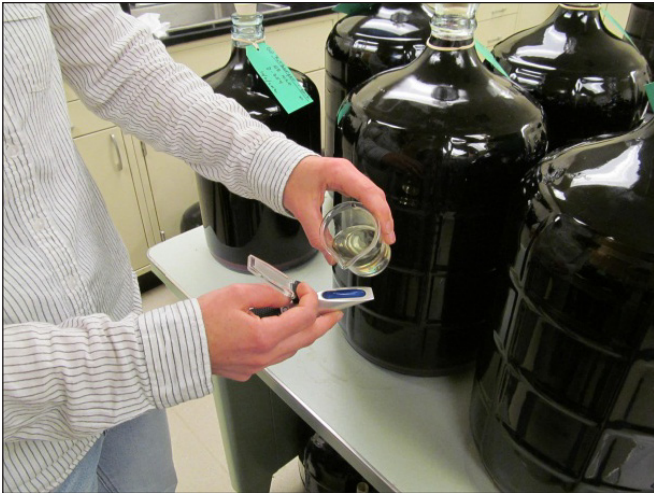
Soluble solids are used to determine optimum harvest time for wine grapes and as an assessment at other points during winemaking.
