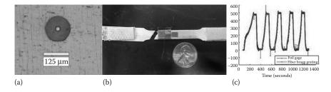
*Figure 17.11* (a) Cross section of fiber optic wire embedded into Al 6061, (b) image of fiber Bragg grating embedded into aluminum and strain gage attached to surface, and (c) comparison of responses of fiber optic sensor and strain gage under a step load input.
