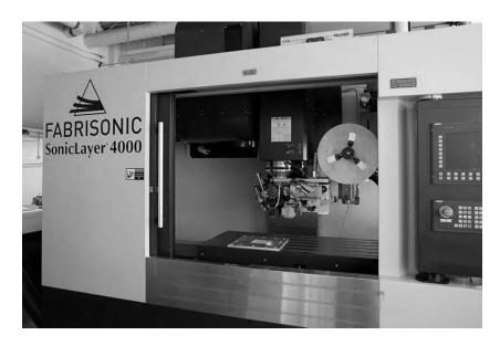
*Figure* **17.3** (See color insert.) State of the art UAM system featuring a 9 kW welder and 20 kN of normal force. This amount of power makes it possible to make high quality, gapless metallic parts.
