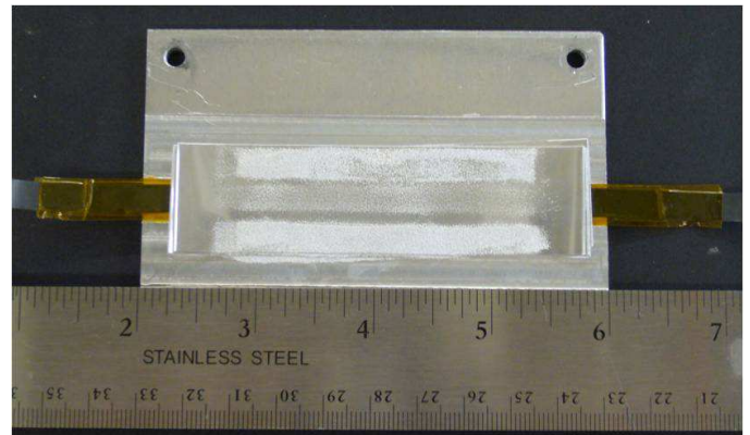
FIGURE 4. 0.102 MM THICK NI-TI STRIP ELECTRICALLY INSULATED BY KAPTON FILM AND EMBEDDED BY UAM INTO ALUMINUM MATRIX.
