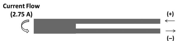
**Figure 3.** Schematic of Ni–Ti strip circuit for resistive heating.
