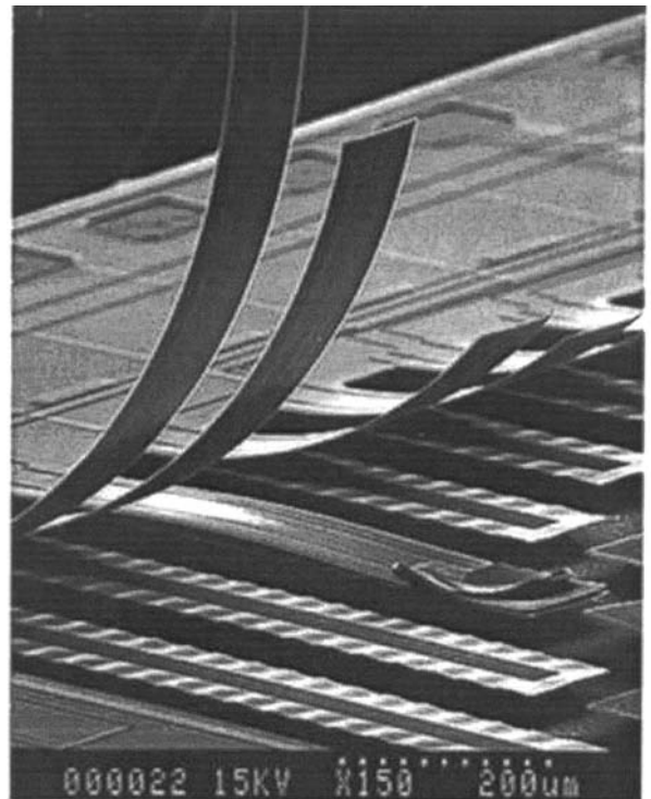
Figure 8 Microcantilever beam used to scale a small mass. The intrinsic interlayer stress will bend the beam. A micromass is used to bend back the beam. The new value of the deflection is directly related to the mass of the microparticle.
