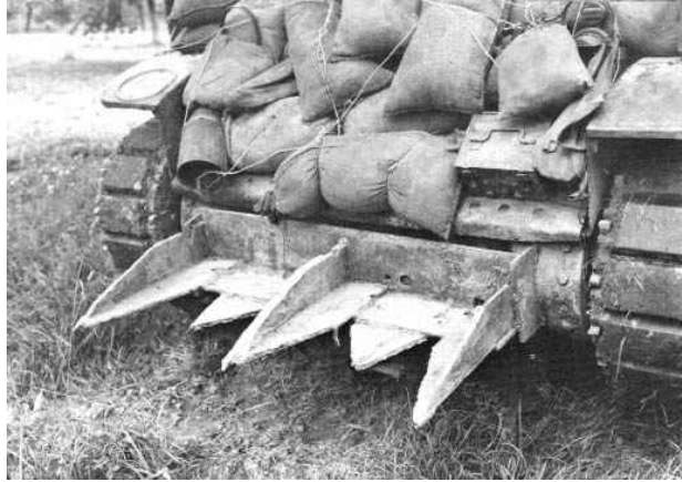
Figure 7. The Culin Hedgerow Cutter is an example of the adapting mode of creativity
