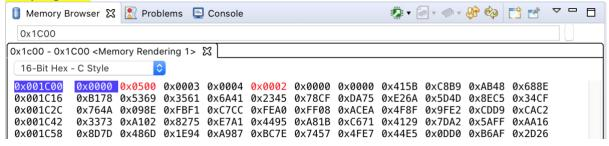
FRAM after entering the debugger by hitting the bug symbol.
