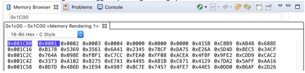
RAM after entering the debugger by hitting the bug symbol, and then running and pausing the program.
