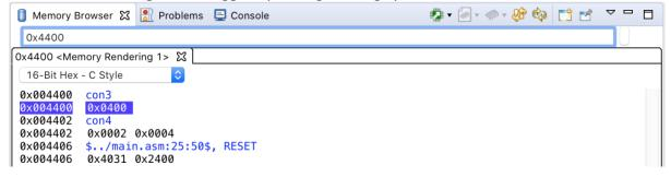
FRAM after entering the debugger by hitting the bug symbol, and then running and pausing the program.
