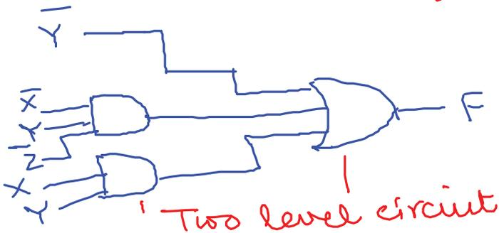
$$\begin{aligned} E(XYZ) &= m_0 + m_1 + m_2 + m_4 + m_5 \\ &= X'Y'Z' + X'Y'Z + X'YZ' + XY'Z' + XY'Z \\ &\quad \text{sum of minterms} \end{aligned}$$
