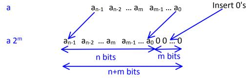
You can safely use an n+m bit bus for a  $x\ 2^m$ . Padding to the left by  $a_{n-1}$  is needed if a wider bus is used
