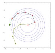
• Since the end isn't moving, we can satisfy the motion constraints by not moving these additional trailers at all. The overall motion then looks like this: the rear of the train isn't moving at all, while the front of the train is moving rigidly. Just one angle is changing.
