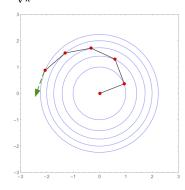
• Observe that the entire train will move rigidly, as if the angles between the successive trailers were welded at certain fixed angle. The last trailer isn't moving; it's just turning.
