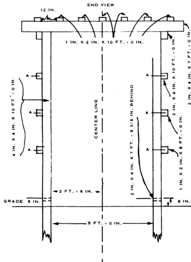
Figure 128. Construction details for a home grape arbor—end view.
