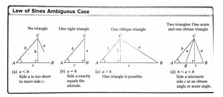
In the above graphic,  $h = b \sin A$  by right triangle trig and **oblique** means "not right."
