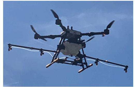
Spray drone with a boom. Photo by Erdal Ozkan, The Ohio State University.
