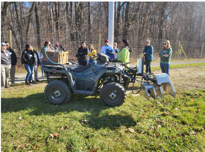
Figure 1. Dr. Sushila Chaudhari (MSU, East Lansing) is conducting studies to test the efficacy and efficiency of smart sprayer technology for weed control in vineyards. The sprayer recognizes the green color of plants and only sprays when it “sees” green.
