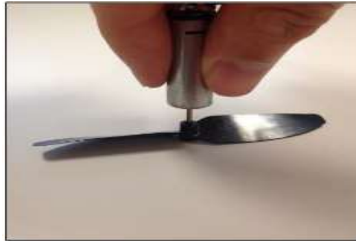
Figure 1: Properly Installing Propeller Onto Motor
