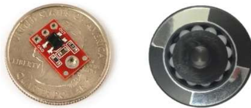
Figure 1. Reflectance Sensor and Wheel with Reflective Tape
