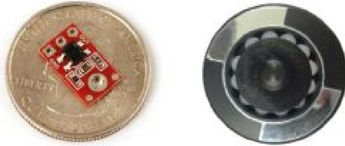
Figure 3: Reflectance Sensor (Left) and reflected taped wheel(Right) 1
