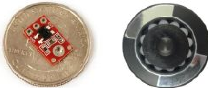
Figure 2: Reflectance Sensor (Left) and reflected taped wheel(Right)
