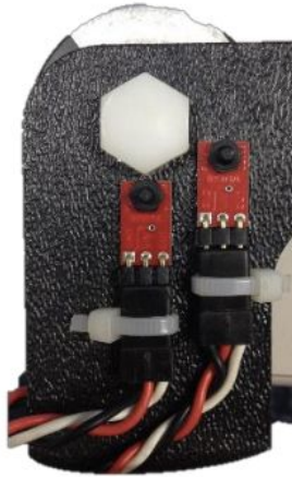
Figure 4: Reflectance Sensors connected to Support Arm
