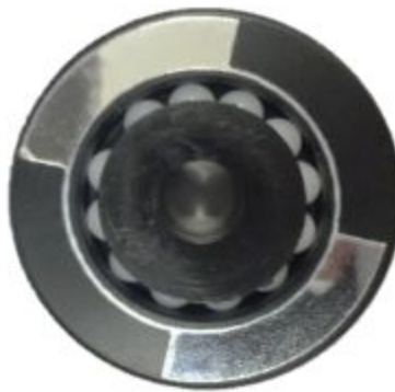
Figure 3: Wheel with Reflective Tape
