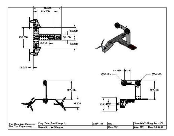
The final T-shape design for the AEV that would be implemented within the experiment. This design allowed for a much more lightweight and stronger build which would assist the AEV greatly in reducing the energy consumed by the AEV.
