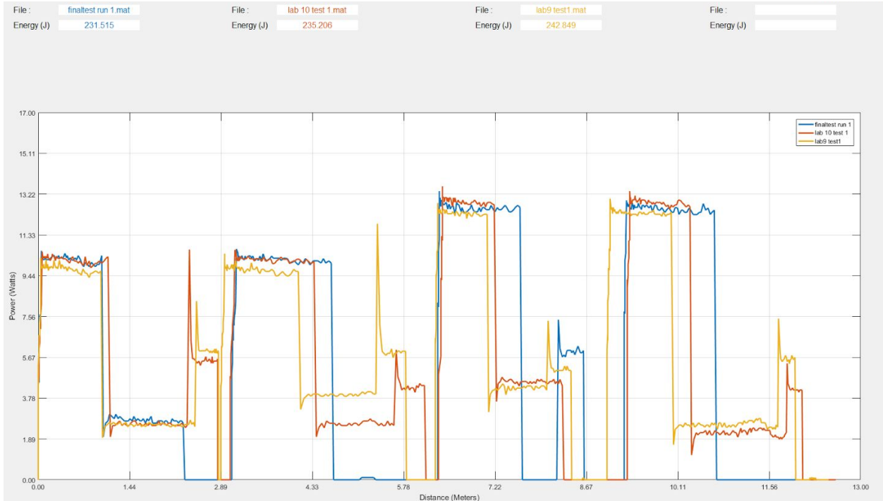
Figure A.15: Power vs. Distance for each of key complete runs of the project. Yellow is the chosen code body from performance test 2, red is the pre-optimization run from performance test 3, and blue is the final run.
