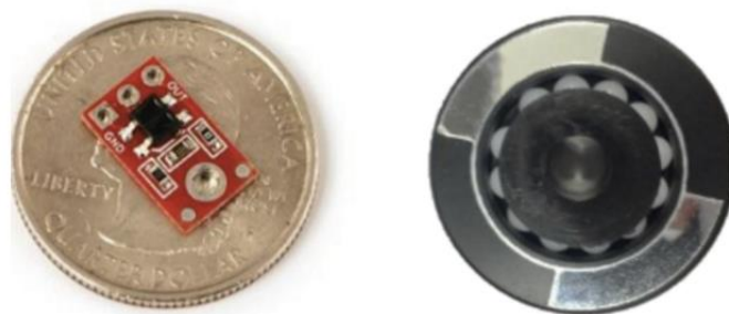
Figure 4: Reflective Sensor (left) and Wheel with Reflective Tape (right)
