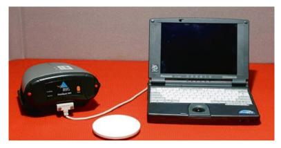
Fig. 13.2 A FieldSpec HandHeld portable spectroradiometer (Analytical Spectral Devices, Denver) (*left*), a reference panel (*middle*), and a laptop computer
