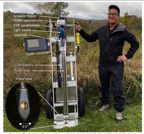
Figure 1. The Subterra Green prototype. Inset: detail of the Subterra Green's probe head.
