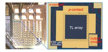
Fig. 2. (Left) Microscope image of fabricated chip imaging the top side contact and electrical probes. (Right) Individual TL array with 11x10 site resonators coupled via link rings at higher magnification.
