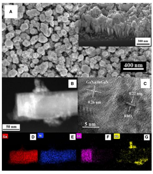
Fig. 2. Characterization of RhO<sub>x</sub>/GaN@InGaN NWs hybrid. a) Front-view SEM image of RhO<sub>x</sub>/GaN@InGaN NW hybrid vertically aligned on silicon. b) Scanning transmission electron microscopy images of RhO<sub>x</sub>/GaN@InGaN NWs at low resolution. c) HRTEM image of RhO<sub>x</sub>/GaN@InGaN NWs. The elemental mapping images of RhO<sub>x</sub>/GaN@InGaN NWs: d) Ga, e) N, f) In, and g) Rh.
