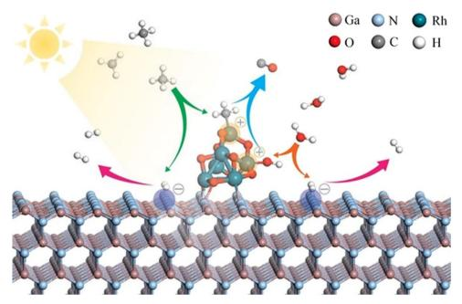
Fig. 1. Schematic for simultaneous adsorption/activation of CH<sub>4</sub> and H<sub>2</sub>O by RhO<sub>x</sub>/GaN system based on DFT calculations.
