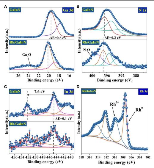
Fig. 3. XPS measurements. High-resolution XPS spectra of a) Ga 3d, b) N 1s, and c) In 3d for GaN@InGaN NWs and RhO<sub>x</sub>/GaN@InGaN NWs and d) Rh 3d for RhOx/GaN@InGaN NWs.
