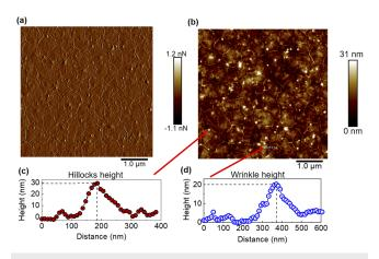
FIG. 4. AFM images of h-BN films under (a) peak force and (b) height scans. The height of the (c) hillocks and (d) wrinkles are also shown.
