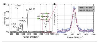
**FIG. 5.** (a) Raman spectra of h-BN films deposited on sapphire substrates, the perturbation corresponding to the  $E_{2g}$  phonon mode is shown as the inset, and (b) a close-up view of the  $E_{2g}$  Raman mode.
