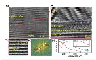
**FIG. 6.** (a) High-resolution cross-sectional TEM image of as-grown 45 ML h-BN films on sapphire, (b) expanded view of the image with the sapphire buffer layer after reconstruction at the growth interface, (c) lattice-spacing of h-BN, (d) FFT pattern of the h-BN cross section, indicating high crystallinity and quality, and (e) EELS spectra of h-BN films confirming sp<sup>2</sup> bonding of h-BN.
