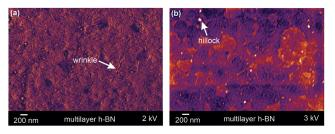
FIG. 3. SEM images of h-BN films, showing (a) wrinkles and (b) hillocks across the surface.
