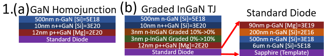
Fig. 1. a) The schematic of the GaN homojunction grown on a standard pn-diode. The GaN homojunction consists of a heavily doped p++GaN/n++GaN junction. b) The schematic of the graded InGaN interlayer tunnel junction which includes a graded InGaN interlayer between the heavily doped p++GaN and n++GaN. In this design a p++ InGaN layer is graded from 0% to 10% In mole fraction on the p-side of the TJ, and a n++ InGaN layer is then graded from 10% to 0% In mole fraction on the n-side of the TJ.
