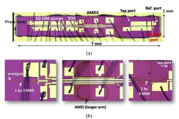
Fig. 13.(a) Photo of the signal-degenerate dual-pumped PSA chip after wire-bonding; (b) close-up views of some sections of the chip.
