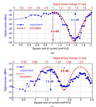
Fig. 26. Comparisons of the measured PSA gain curve and the theoretical simulation. (a) one-period PSA gain curve with 6.3 dB experimental and 6.5 dB theoretical results; (b) two-period PSA gain curve with 7.8 dB experimental and 8.5 dB theoretical results.
