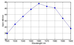
Fig. 8.Measured wavelength-dependent small-signal gain profile
