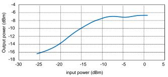
Fig. 9. Measured output power of the SOA with respect to the input power
