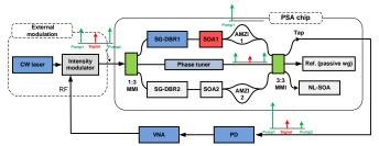
Fig. 19.Relative signal phase measurement setup.
